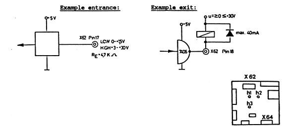
3. To plug X64/PIN 5,6 an opener contact can be connected, with same function as X62/PIN 10 (e.g. function end guard of door). h3 lights up when door is open (J4).
